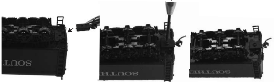
Insert the coupler (as shown) and screw into place
