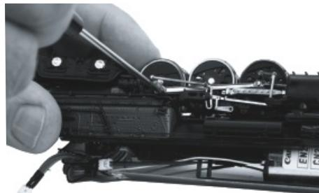
MAKE NOTE OF THE ECCENTRIC CRANKS IN REALTION TON THE AXLE IF THE DRIVER BEING CHANGED. THE ECCENTRICS MUST BE RE-ASSEMBLED IN THE SOME POSITION.
