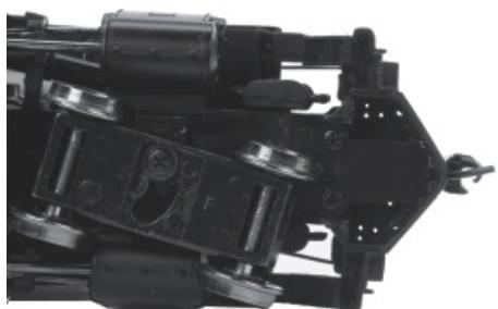
Engine Coupler Installed Underside View
