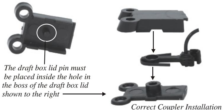
Now mate the draft box lid and coupler with the draft box. The pin on the inside of the draft box mates with the hole in the boss of the draft box lid. When mating the draft box and the lid, make sure that the whisker springs on the coupler are inside of the draft box.
