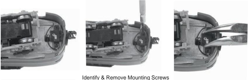
Identify & Remove Mounting Screws
