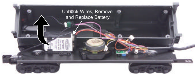
Figure 9. Replacing the Battery
