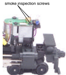
Figure 6. Smoke Unit Inspection Cover
