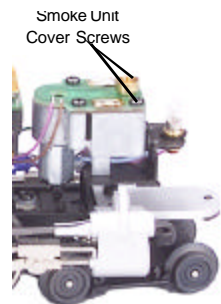
Figure 6. Smoke Unit Inspection Cover
