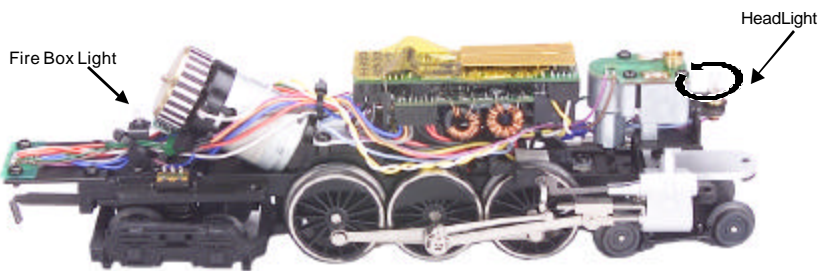
Figure 7. Replacing the Headlight and the Fire Box Light
