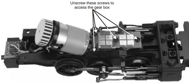
*Figure 7. Motor Gearing Plate Screws*
