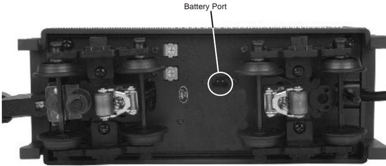
*Figure 10. Battery Recharging Jack*
