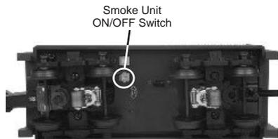
Figure 2. Smoke Unit Switch Location
