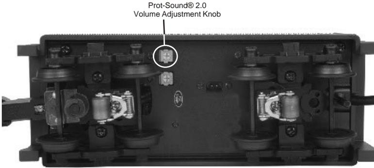
*Figure 4. Manually Adjusting The Volume*
