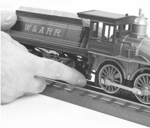
Figure: Attaching the Plastic Drawbar Holder
