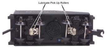
Figure 2. Lubrication Points on the Tender
