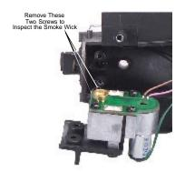
Figure 8. Inspecting the Smoke Unit's Wick
