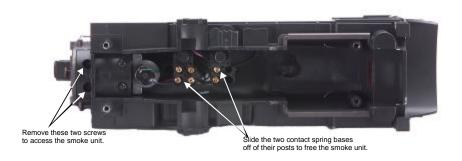
Figure 7. Removing the Smoke Unit Mouting Plate to Access the Smoke Unit
