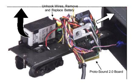
Figure 11. Replacing the Battery
