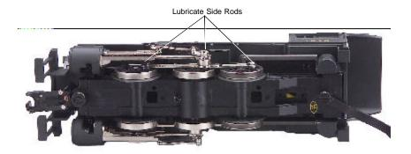
Figure 3. Lubrication Points on the Engine
