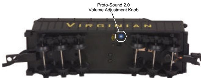
Figure 1. Proto-Sound 2.0 Volume Adjustment Knob
