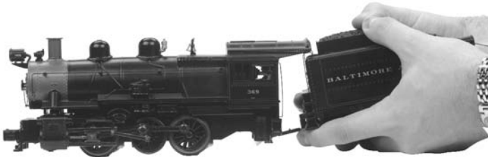
Fig. 4: Connecting Locomotive to Tender
