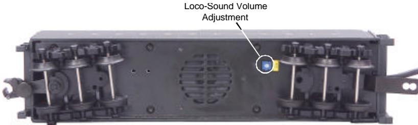
*Figure 1. Loco-Sound Volume Adjustment Knob*
