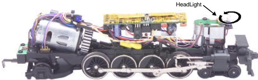
Figure 7. Replacing the Headlight
