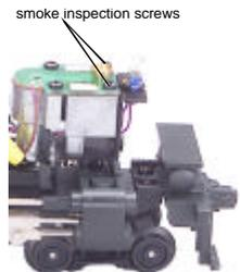
Figure 6. Smoke Unit Inspection Cover
