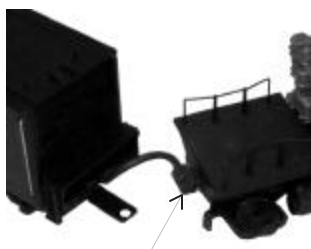
Plug Tender Plug Into Boiler Socket At Back Of Cab
