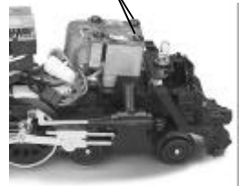
Figure 6. Smoke Unit Inspection Cover
