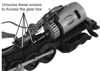
Figure 10: Motor Gearing Grease Plate Screws
