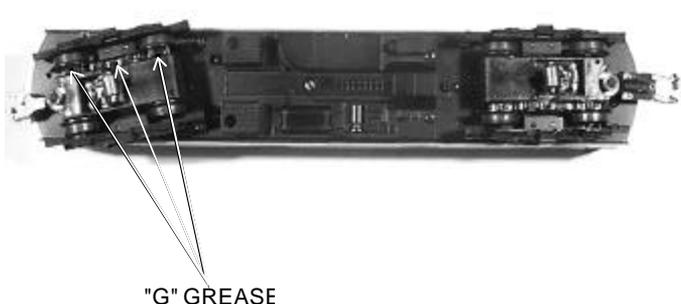
Figure 4: Lubricate The Truck Bushings
