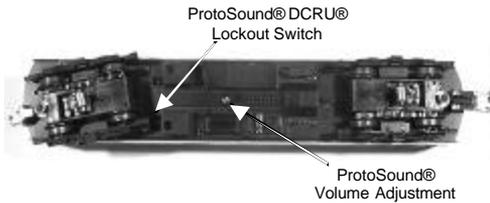
Figure 1: Locating The Powered Subway Car's switches
