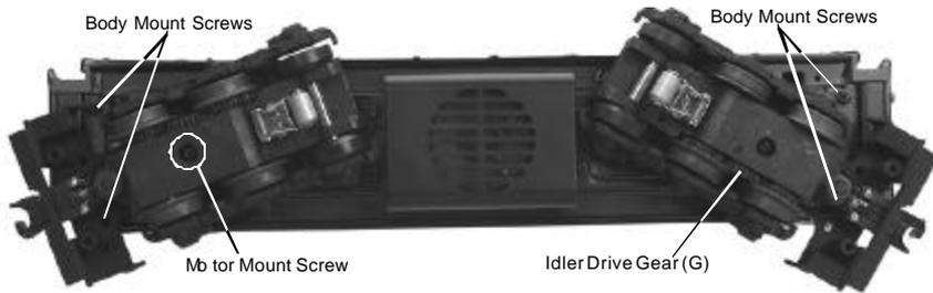
Figure 3. Lubrication Points on the Engine
