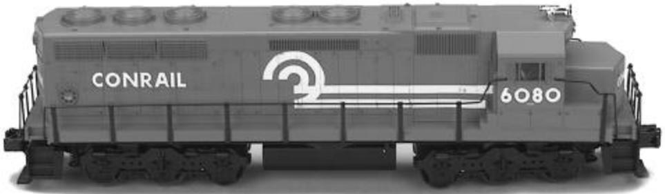
The RailKing SD45 is a model of a 3600HP Mainline Freight Locomotive. It has an ABS body and stamped metal floor and runs on O-31 track. This RailKing Diesel Engine contains M.T.H.'s Loco-Sound™ sound and train control system. The locomotive is easy to operate with any compatible standard AC transformer (see the compatibility chart on page 14), and is completely compatible with most other 3-rail locomotives, rolling stock, and accessories.
