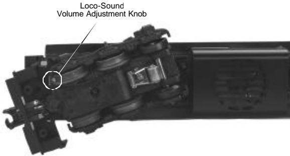
*Figure 1. Location of the Loco-Sound Volume Adjustment Knob*
