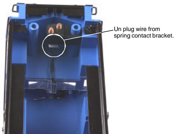
Figure 5. Location of the headlamp in the Engine.
