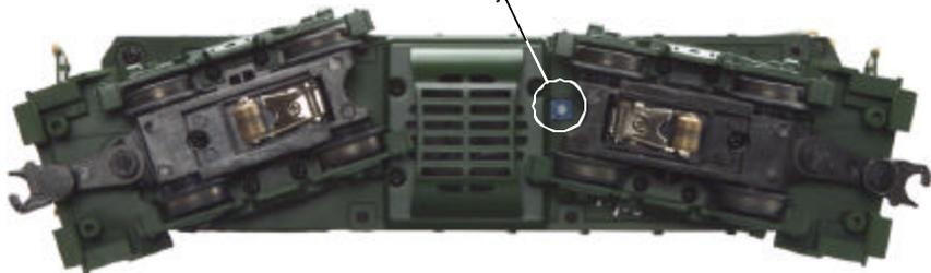
*Figure 1. Location of the Loco-Sound Volume Adjustment Knob*
