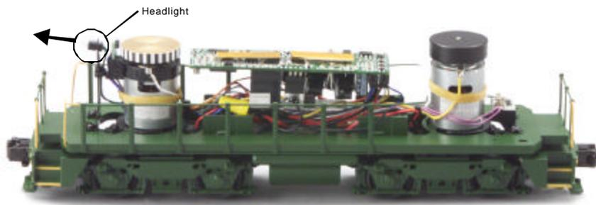
*Figure 5. Location of the headlamp in the Engine*
