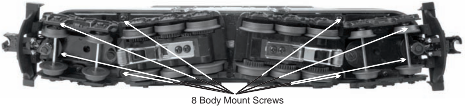
Figure 9: Removing Body Mount Screws
