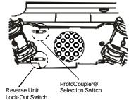
Figure 1: Lock-Out Switch Location
