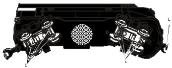
Figure 6: Lubricating The Locomotive Chassis
