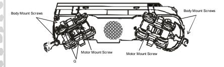
Figure 7: Lubricate The Tender Chassis Trucks
