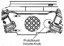
Figure 4: Adjusting The ProtoSound Volume
