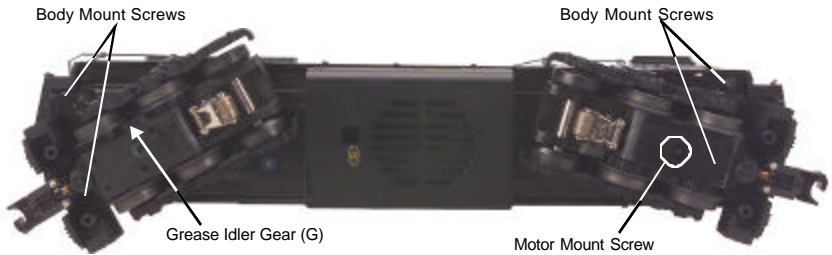
Figure 3. Body Mount Screws and Greasing Points.
