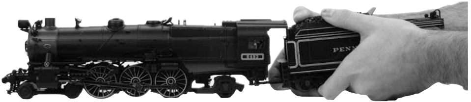
Figure 5: Connecting Locomotive to Tender
