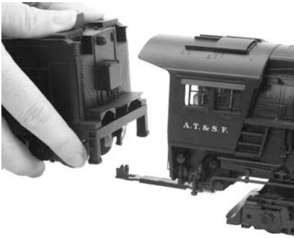
Figure: Connecting Locomotive to Tender
