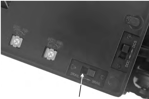
Power Input Switch
