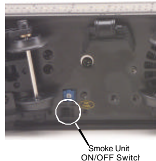
Figure 4. Smoke Unit ON/OFF Switch
