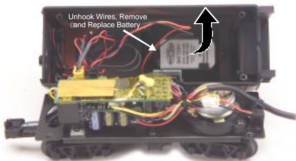
Figure 11. Replacing the Battery
