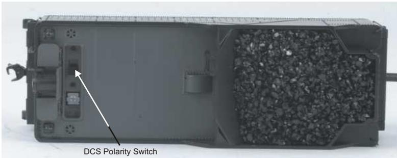
Figure 4: Changing the polarity with the locomotive polarity switch
