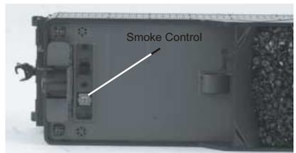
Figure 9: Smoke Unit Switch Location (Inside Tender Hatches)
