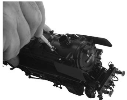
Figure 5: Installing Smoke Deflectors
