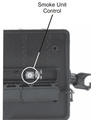
Figure 2: Smoke Unit Control Location
