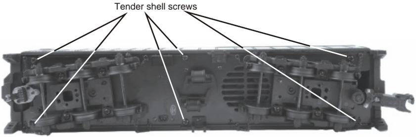
Figure 9: Tender Shell Screw Location
