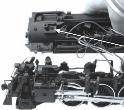
Remove screw to free smoke unit. Then turn smoke unit over to inspect.
