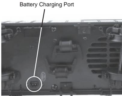
Figure 11: Battery charging port Location
