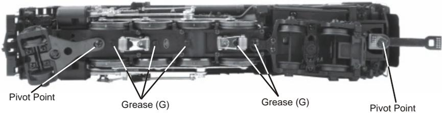
Figure 5: Lubricating the grease points
