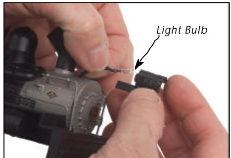
*Figure 8 - Replacing the Headlight*
