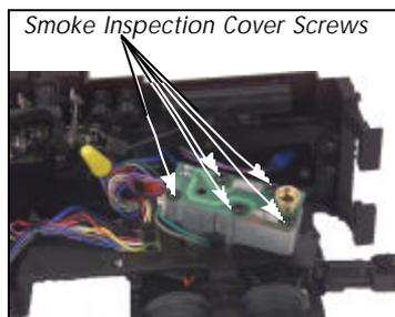
Figure 6 - Smoke Unit Inspection Cover
