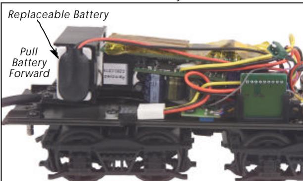
Figure 10- Replacing the Battery
