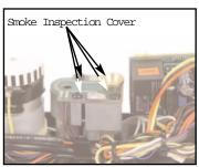
Figure 7 - Smoke Unit Inspection Cover
