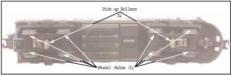
Figure 2 - Lubrication Points on the Engine
