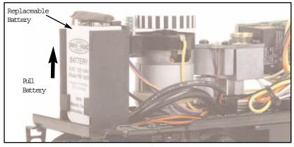
Figure 11- Replacing the Battery
