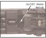
Figure 6 - Smoke Unit On/Off Switch
