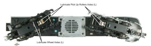
Figure 1. Lubrication Points on the Locomotive
