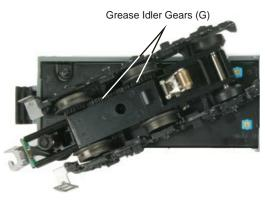
Figure 7. Greasing The Idler Gears
