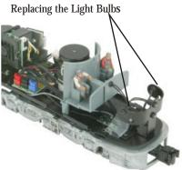
Figure 8. Replacing the Light Bulbs
