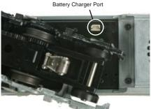
Figure 9. Battery Charger Port location.
