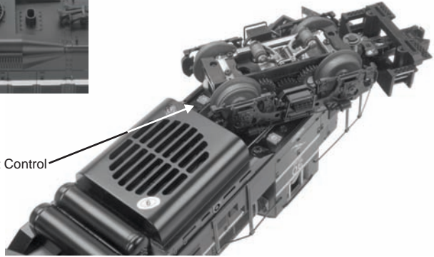
Figure 3: Smoke Unit Control
