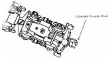
Figure 3: Lubricating The ProtoCoupler Knuckle
