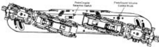
Figure 2: Locating The Proto-Coupler® Selection Switch
