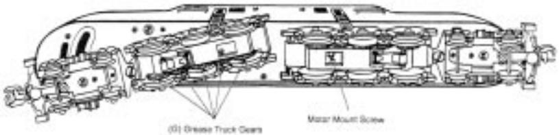
Figure 8: Greasing The Power Trucks
