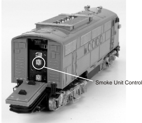
Smoke Unit Control
