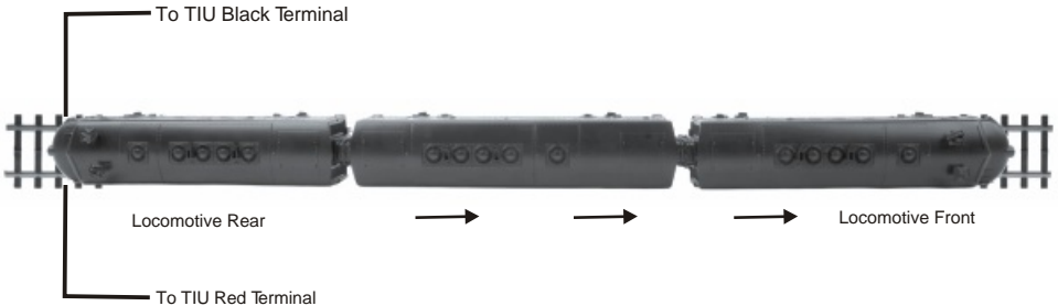
Proper 2-Rail Polarity wiring and locomotive orientation
