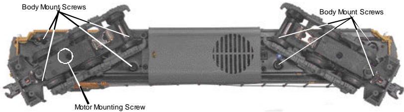
Figure 5: Body Removal Screw Locations
