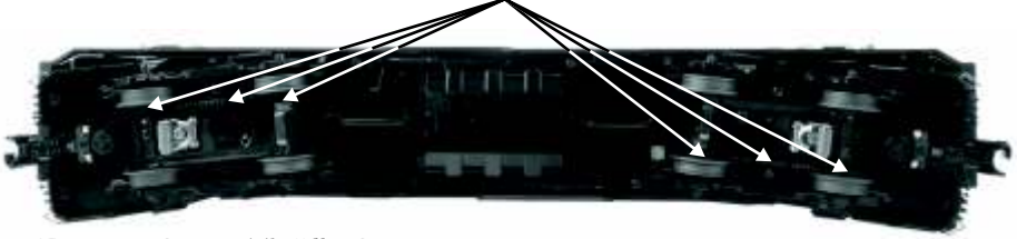
Figure 10: Greasing The Idler Gears
