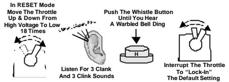
time to check each RESET feature one at a time. To reset all the RESET features back to their original factory settings, enter RESET and go to Feature 18. (See the section entitled *Using RESET To Program ProtoSounds®* on page 18). Once in Feature 18, press the transformer whistle button and wait for ProtoSounds® to sound a garbled bell sound. Then interrupt the throttle to enter forward.
