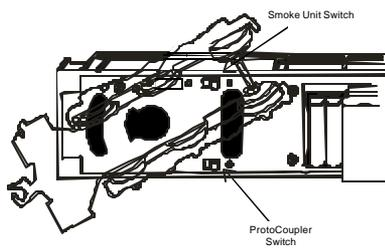
Figure 1: Locating The Smoke Unit Switch and ProtoCoupler Switch.
