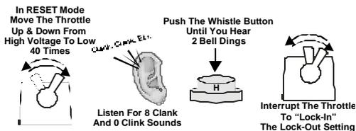
the way off and then back on again. To turn the Remote Lockout Control setting back off, go back to Feature 40 and press the whistle button until only one bell ding sounds. To lock in the setting, simply turn the transformer throttle off and then back on again. Alternatively, you can go to RESET Feature 18 to reset all ProtoSound® features back to their original factory defaults including Remote Lockout Control.
