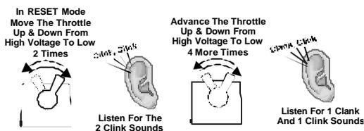
times the throttle is advanced by playing back the number of “Clinks” and “Clanks” to confirm the feature you’ve selected.
