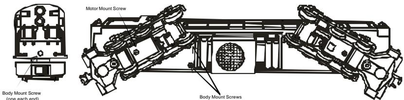
Figure 8: Removing The Body From The Chassis
