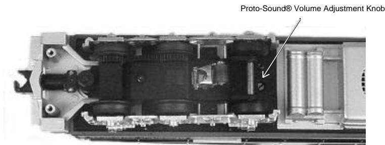
*Figure 4: Adjusting The ProtoSound® Volume and selecting the ProtoCoupler*
