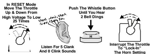
ProtoSounds® has been programmed to sound the horn in neutral). Turn the throttle off and then on again to “Lock-In” your selection. Now, whenever you are in neutral, you can blow the horn with the transformer whistle button. To reset ProtoSounds® to its original factory setting of no horn in neutral, repeat the above procedure but keep pressing the whistle button in Feature 25 until ProtoSounds® only dings once instead of twice.
