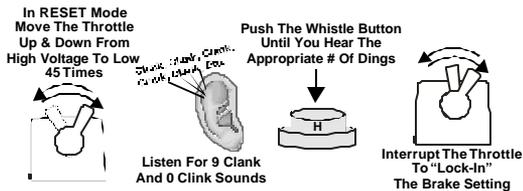
then on again to "Lock-In" the new setting. To reset the computer to its original factory default setting (option 2 - squeaking brakes are activated for full-time operation), repeat the above procedure but keep pushing the whistle button until the module only responds with two bell dings.
