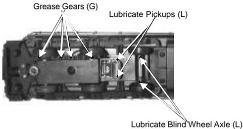
Figure 6: Lubricating The Locomotive Chassis
