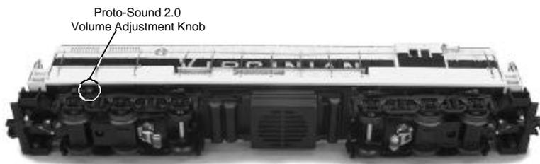
*Figure 1. Proto-Sound 2.0 Volume Adjustment Knob*
