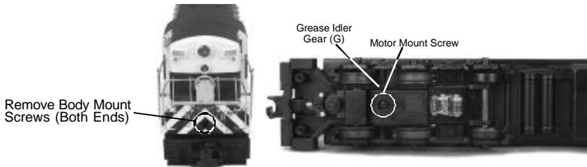
Figure 6b. Second Set of Body Mount Screws
