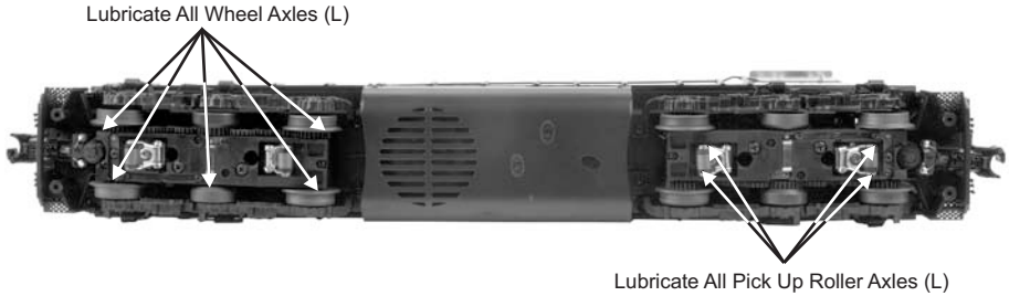
Figure: Lubrication Points on the Locomotive
