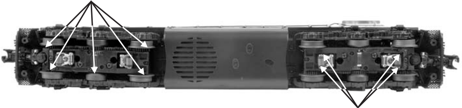
Figure: Lubrication Points on the Locomotive
