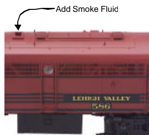
Figure 3. Add Smoke through the Front Smokestack
