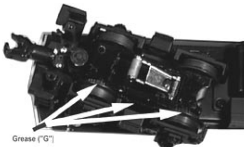
Figure 8: Greasing The Power Trucks
