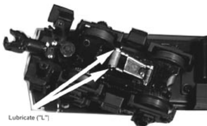
Figure 7: Lubricating The Pickup Rollers
