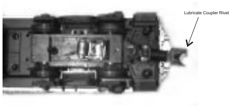
Figure 3: Lubricating The ProtoCoupler Knuckle
