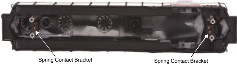
Figure 10. Replacing the Lights Mounted on the inside of the Shell
