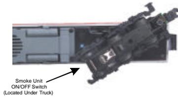
Figure 3: Smoke Unit Switch Location
