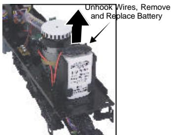
Figure 10: Removing the battery
