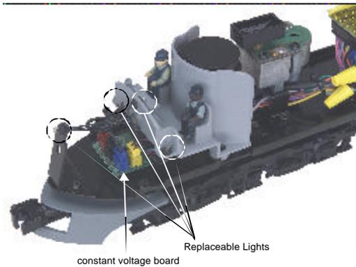
Figure 8: Replaceable light bulb locations
