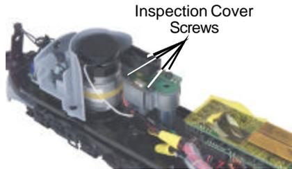
*Figure 12: Inspecting The Smoke Unit Wick*
