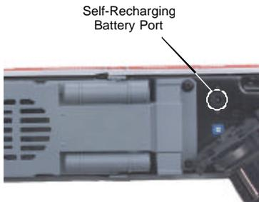
Figure 9: Battery recharging port
