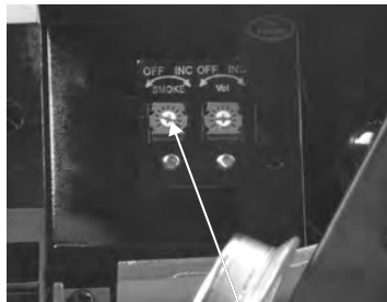
Smoke Unit Control
