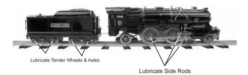
Lubricating The Side Rods and Linkage and tender wheels and axles
