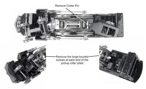
•Lubricate the Drive Gear and Worm Gear with White Lithium Grease. Make sure when replacing Contact Plate that the Plunger Pin makes contact with the Flat Contact plate.
