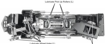
Lubricate Wheel Axles (L)
