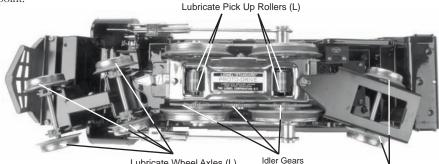
Lubricate Wheel Axles (L)
