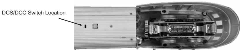
Figure 7: Changing from DCS to DCC Mode
