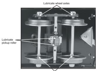
Lubricate where axle meets wheel and where axle meets truck side.
