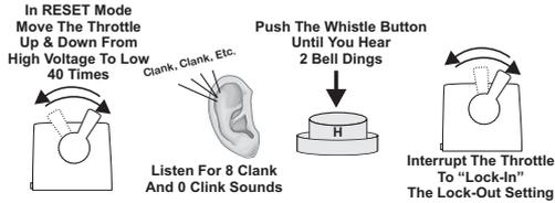
To lock in the setting, simply turn the throttle all the way off and then back on again. To turn the Remote Lockout Control setting back off, go back to Feature 40 and press the whistle button until only one bell ding sounds. To lock in the setting, simply turn the transformer throttle off and then back on again. Alternatively, you can go to RESET Feature 18 to reset all ProtoSound features back to their original factory defaults including Remote Lockout Control.
