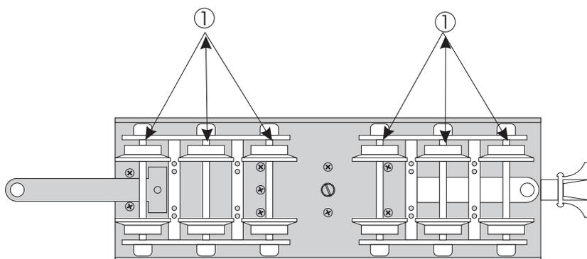
*Figure 8: Removing The Boiler From The Chassis*
