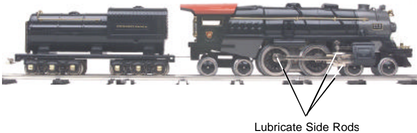
Figure 2: Lubricating Side Rods
