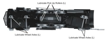
Lubrication Points on the Locomotive
