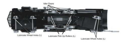
The locomotive utilizes a direct drive motor that should not need direct lubrication. However, it will be necessary to lubricate the idler gears located on the inside of the drive wheels.
